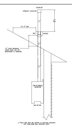
\*\*IMPORTANT NOTE: All vent pipes must be glued, properly supported, and the exhaust must be pitched a minimum of a ¼" per foot back to the heater (to allow drainage of condensate).
